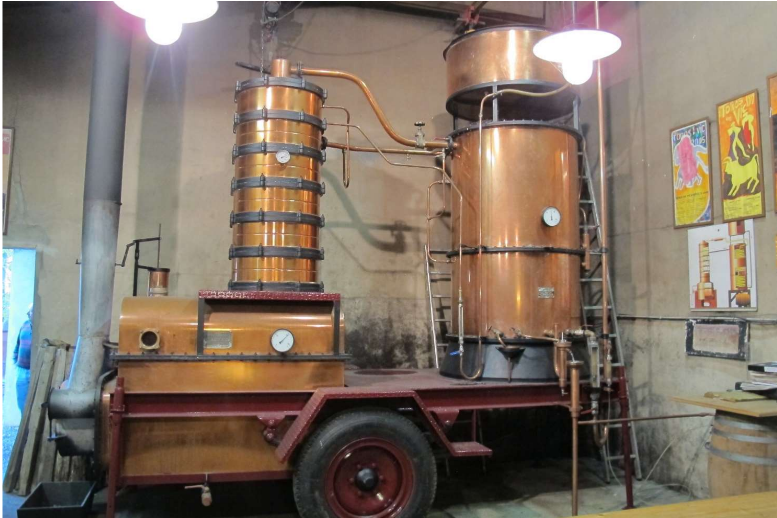
Mobile wood-fired copper Armagnac still (single distillation)
