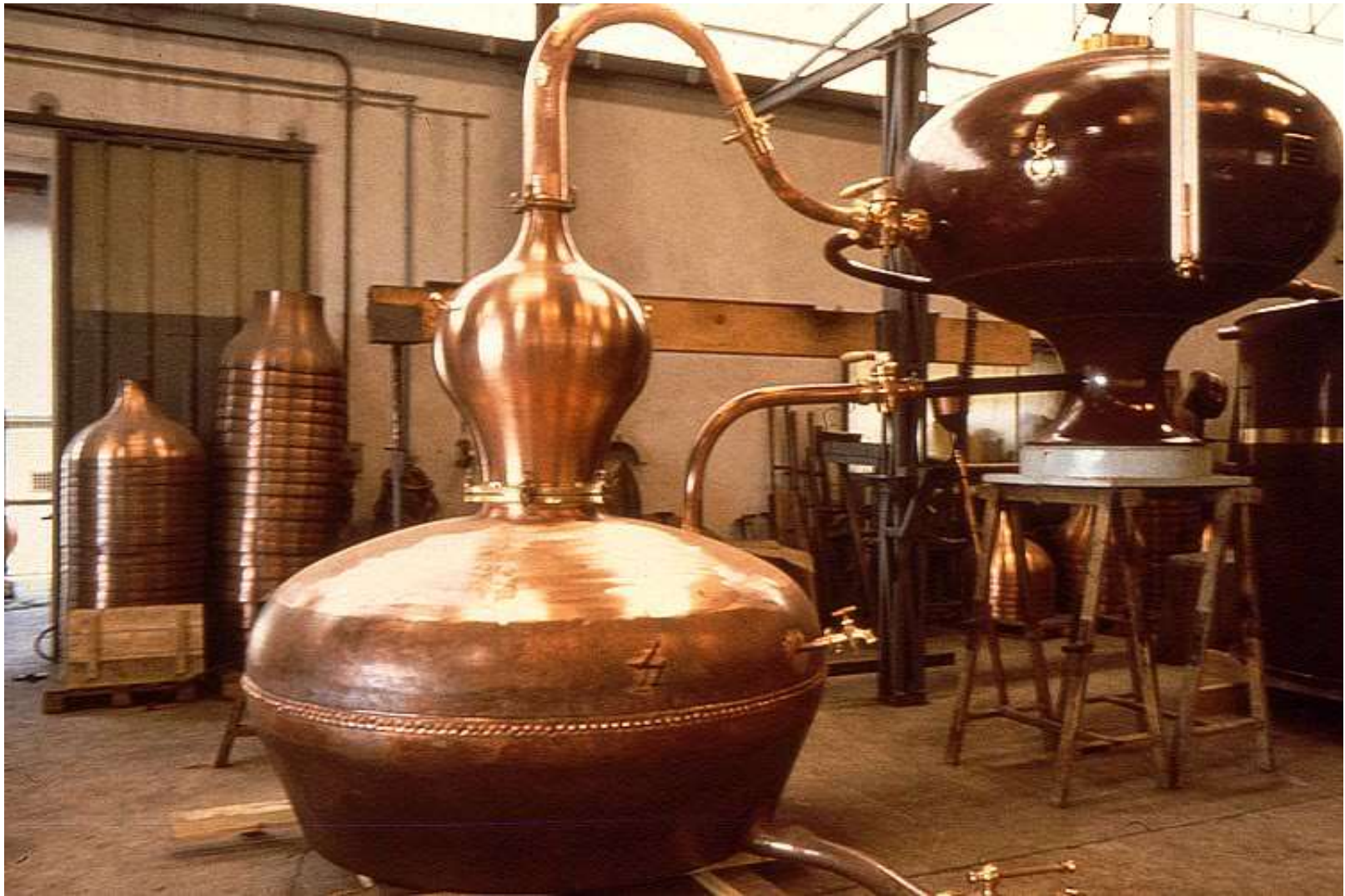
Copper Cognac Alambic Still (double distillation)
