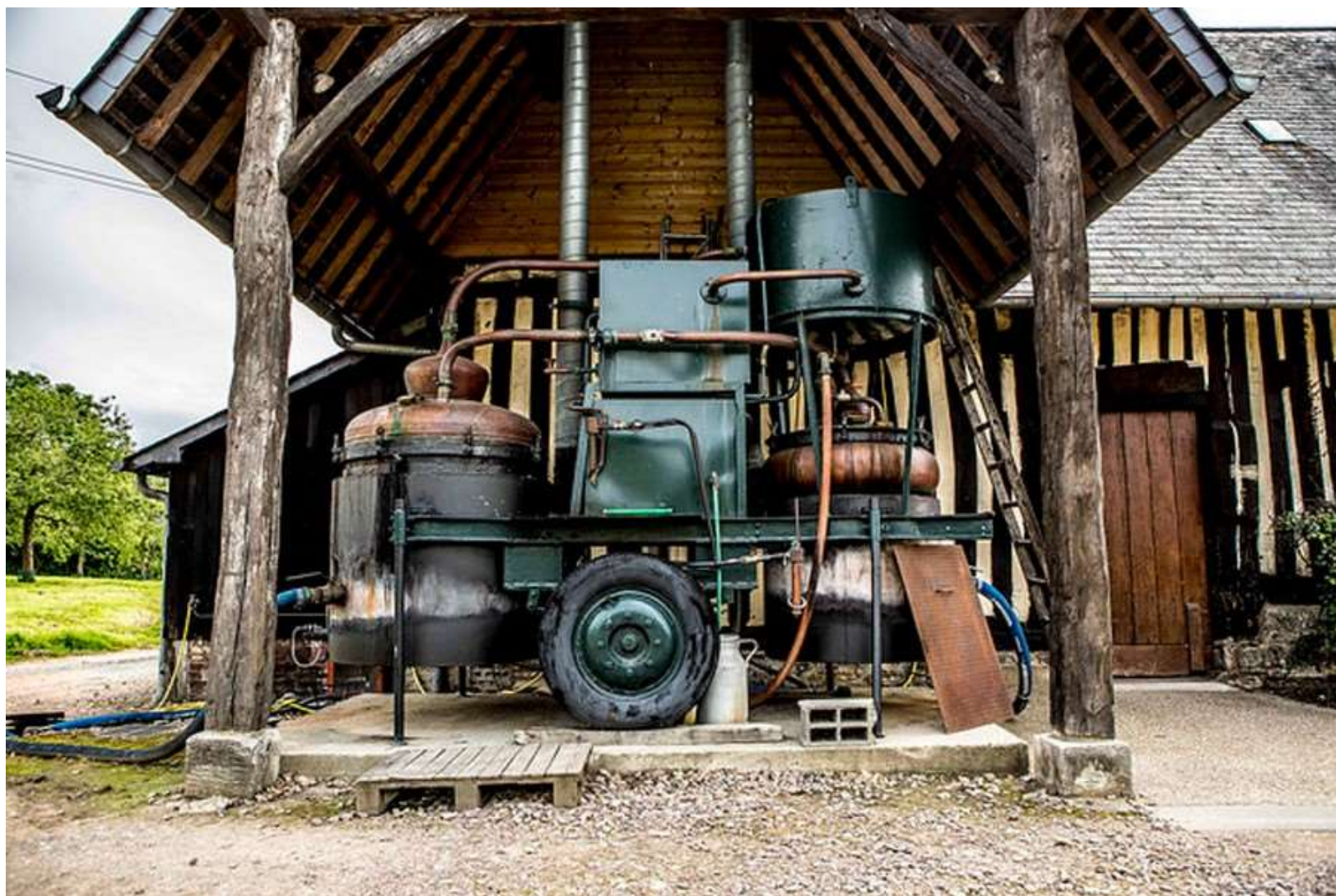
Semi-mobile Calvados still (double distillation)
